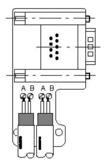
1: The bus cable can be connected to either the left or right set of terminals!
