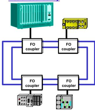
Fiber optic segments enable redundant wiring
