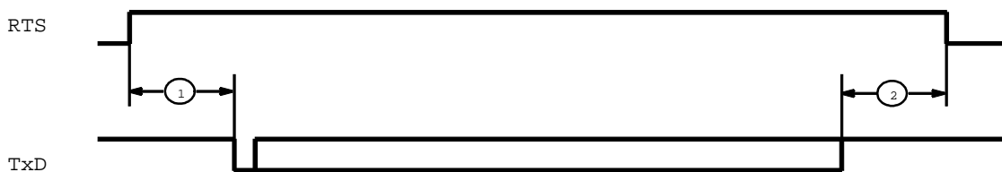
Figure 9.6-3: Transmit Timing, XCTS constant log. '0'
