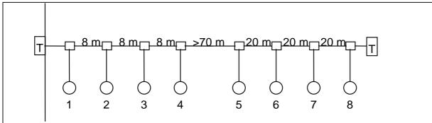
Decoupling element between stations 2 and 3, 5 and 6, 6 and 7, 7 and 8
