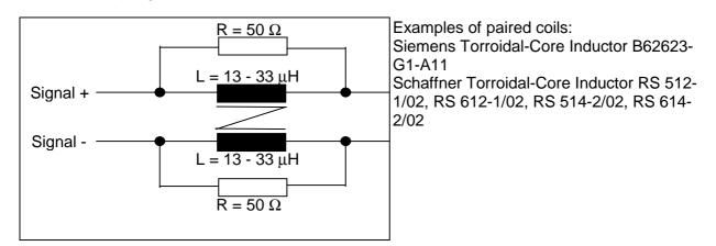
Example of a decoupling element:
