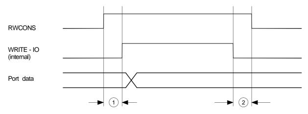
**Read timing:** The user can freeze external latches for instance with RWCONS in order to accept consistent data at the ports programmed to Input ("Snapshot" option).
