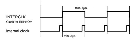
A read access operation takes 200  $\mu$ s for one complete read cycle. A write cycle requires 100  $\mu$ s, in addition to the programming time of approx. 10 ms per word.
