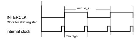
The shift register controller operates with the same clock frequency as the EEPROM controller, i.e. 250 kHz. A read access operation takes  $96 \mu s$ .
