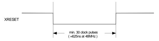
A flip-flop series is integrated upstream of the reset logic. This filter filters noise spikes up to a length of 8 XTAL1 clock periods in order to prevent interference on the RESET line.
