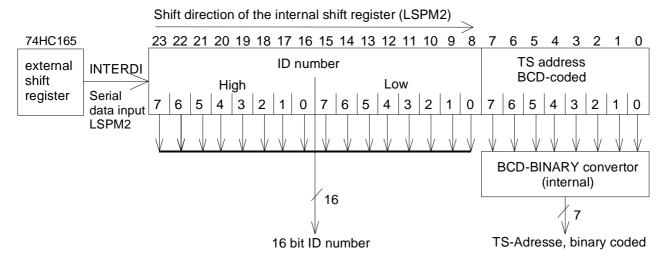
A total of 24 bits must be stored in the external shift register: 16 bits for the ID number and 8 bits for the TS address.
