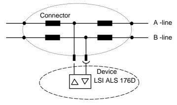
The following line parameters were used for dimensioning the length inductors of L = 120 nH based on the following assumptions:
