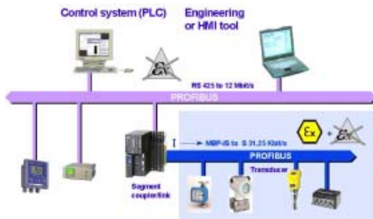
Fig. 19: Plant topology and bus powering of field devices using MBP transmission technology
