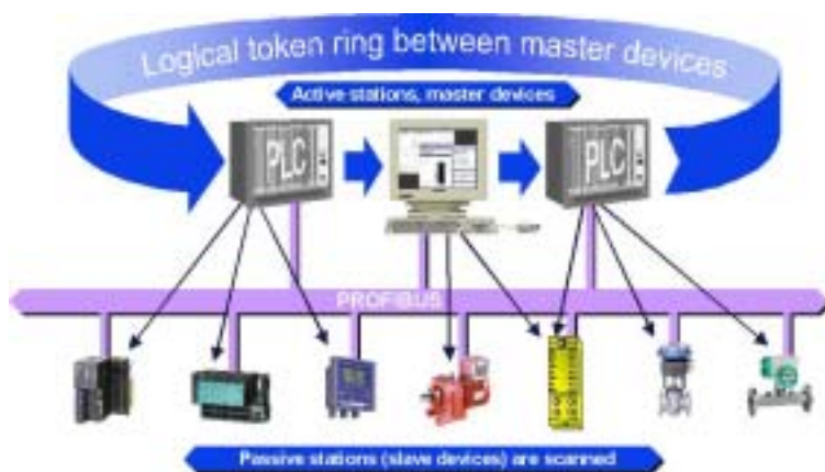
Fig. 6: PROFIBUS configuration with active masters and slaves
