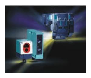
The IQ -Sense module for the Simatic ET 200S distributed I/O system from Siemens. lets you coordinate photoelectric sensor parameters, such as sensitivity, output selection, function, and hysteresis, over PROFIBUS DP. The module snaps into an ET 200S station and coordinates parameters from a sensor s 2-wire cable. Setting -up can still be performed manually at a sensor s teach-in button. IQ-Sense features full PROFIBUS DP diagnostics.
