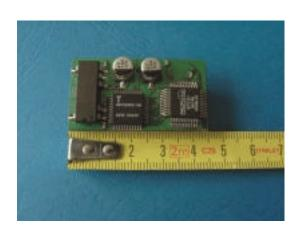
UNIGATE-IC is a low-cost miniature PROFIBUS gateway 'that is small enough to be integrated into components such as intelligent sensors. It includes all digital and analogue PROFIBUS functions and enables users to implement PROFIBUS connectivity with minimum effort and fieldbus knowledge. The module has a hybrid structure and uses a standard PROFIBUS chip for full compatibility with the spec. A Protocol Developer tool aids program development.
