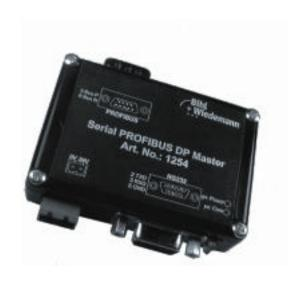
The new Serial PROFIBUS Master is a commissioning and service tool for PROFIBUS DP and PROFIBUS PA slaves. It can scan a network for connected slaves, exchange I/O data with a slave in cyclic mode and display the diagnostics. PROFIBUS DP slaves can also be operated in the DP-V1 acyclic mode, which is helpful for commissioning complex field devices like drives, modular I/O and PROFIBUS PA slaves. It can work as a Class 2 Master.
