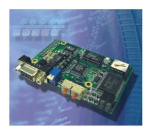
The AnyBus family of embedded communication modules now includes a module for DP-V1 support. It is hardware and software backwards-compatible with
