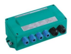
Up to 31 instruments can be connected to a single PROFIBUS PA segment using Fieldbarrier, which allows non-IS Segment couplers to power instruments in hazardous locations. Fieldbarrier has 4 FISCO IS outputs, and 4 PROFIBUS PA instruments can be connected to each over a bus length of 120 metres.
