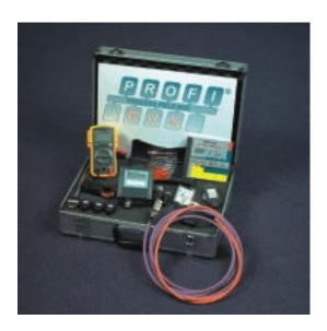
PROFIBUS Center Nederland together with Endress + Hauser have developed a First-aid kit for maintenance specialists. It is intended for the analysis and resolution of **PROFIBUS** common malfunctions. Maintenance specialistes introduced to the kit have been overwhelmed by the completeness of the kit, apparently.
